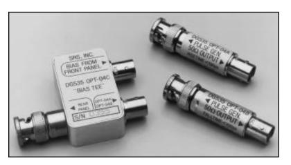
Therefore some accommodation must be made to provide a DC current to forward bias the SRD prior to the output pulse. This current is applied via a "bias tee" (Option 04C) which passes the bias current through an inductor to the diode. The same inductor prevents the pulse from the rear panel output from passing to the bias source. A front panel output may be used as the bias source.
